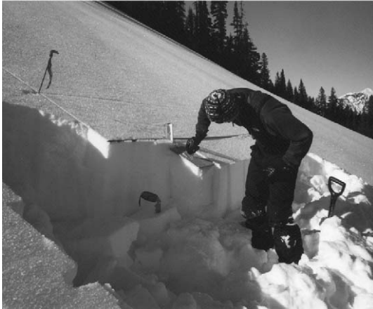
Fig. 2. A surface mode QLCT being performed during the 27 Jan. 2001 stability-sampling trials at the Bradley Meadow site in the Bridger Range, MT. The observer is applying a rapid vertical load to a 0.08 \text{ m}^2 isolated column of snow at the centroid of a plywood load plate using a mechanical force gauge (Landry et al., 2001).
