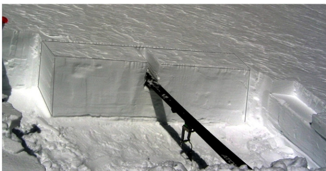
Fig. 5. CECT experiment. The test sample (contour enhanced) is cut free from the surrounding snowpack. A small trench of variable depth and fitting the ski is dug into the center of the sample. Fracture in the weak layer is initiated by tapping on the ski.
